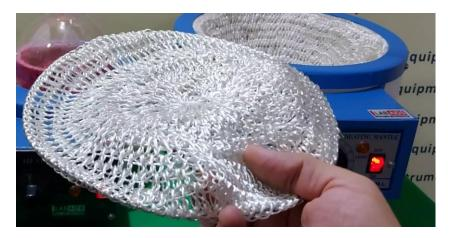
Glass wool Insulation is provided between the walls to prevent the exterior from over-heating. These heating mantles operate on 220V, 50Hz AC and are available in 250ml, 500ml, 1000ml, 2000ml, 3000ml, 5000ml, 10 Ltrs., and 20 Ltrs. Capacities. Spare heating mantles / elements are also available.
